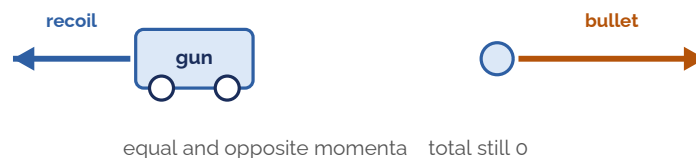
Fig 9.2 — Recoil: before firing the total momentum is zero; afterwards the gun and bullet carry equal and opposite momenta.
