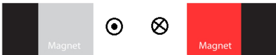
Motor coil cross-section: dot/cross shows force direction on each side
