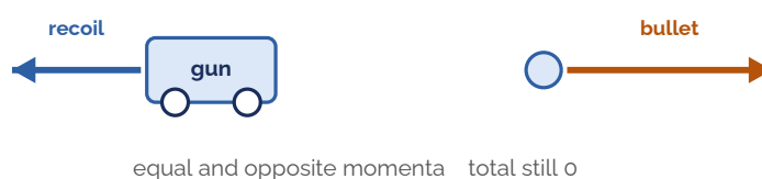
Fig 9.2 — Recoil: before firing the total momentum is zero; afterwards the gun and bullet carry equal and opposite momenta.
